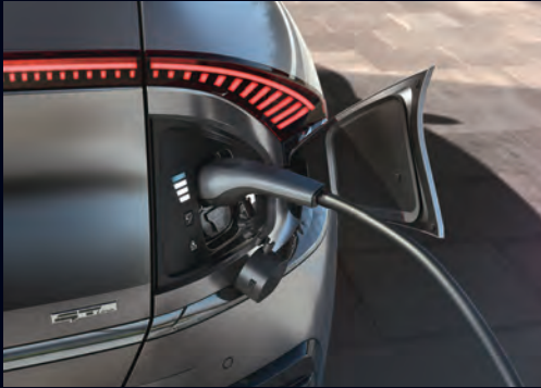
Ultra-fast Charging With 800V ultra high-speed charging capability, the Kia EV6 takes as little as 18 minutes* to charge from 10% to 80% *With 350kW charger
