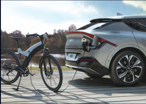
Vehicle-to-Load (V2L) Fully charged, EV6 offers 3.6 kW of power to run multiple devices inside and outside by attaching Vehicle-to-Load connector
